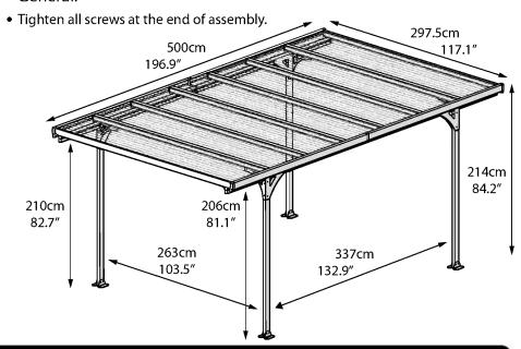
Do not tighten screws and nuts (411 & 412) until completion of assembly process. These 2 icons indicate if screws' tightening is required or not.
