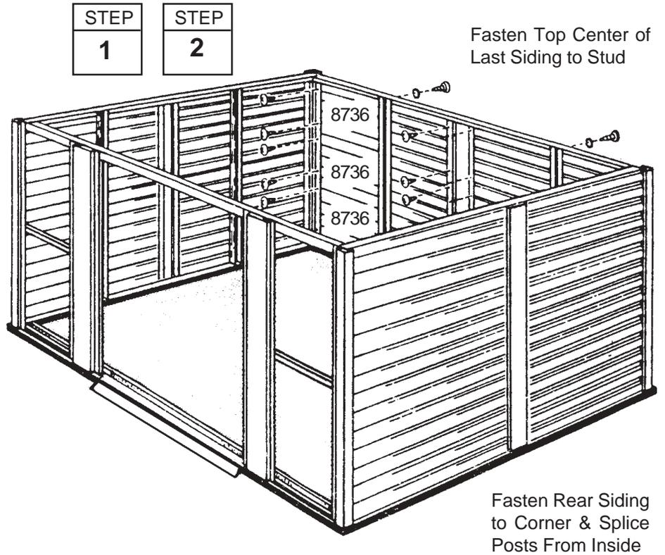
**3** Slide **front siding** into channels of corner post and door jamb. This siding is fastened from the inside, using screws into post and jamb.
